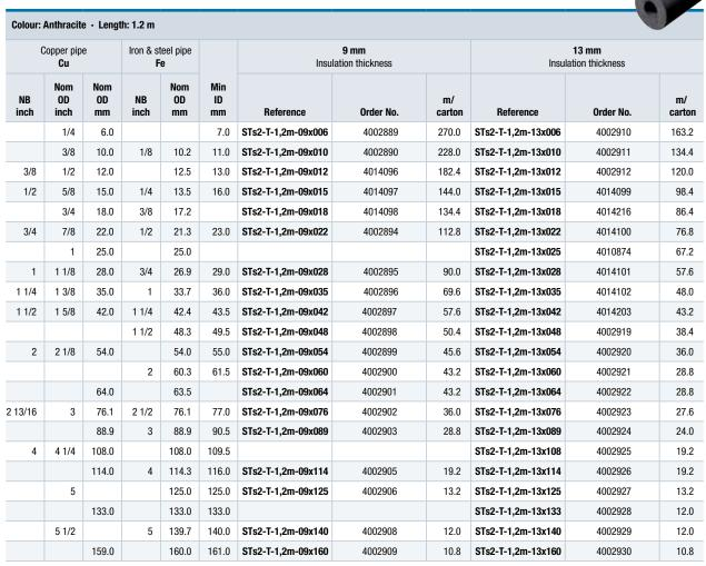
All tubes are available as slit items. For ordering slit items add "-SL" to the reference codes above (example: STs2-T-1,2m-13x076-SL).
